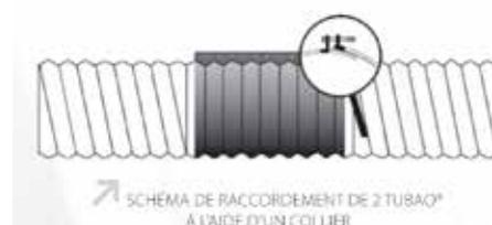
SCHEMA DE RACCORDEMENT DE 2 TUBAO® A L'AIDE D'UN COLLIER
