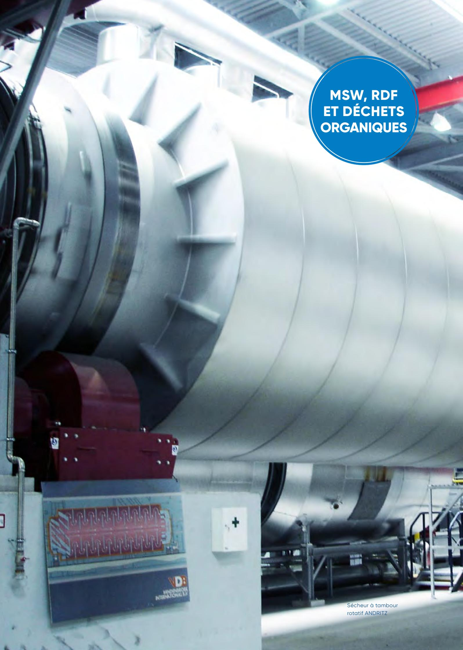
A large, horizontal, stainless steel rotary drum dryer is the central focus of the image. The drum is supported by a complex metal structure and has several large, curved blades or paddles attached to its exterior. The background shows an industrial facility with overhead pipes and structural beams. In the foreground, there is a control panel with a red emergency stop button and a white electrical box with a green cross symbol. A technical drawing of the drum is mounted on the control panel.
